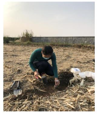
Fig. 2.4. Soil sampling for bulk density definition
