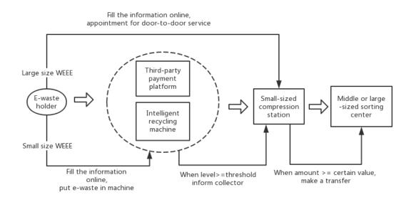
Figure 1.8 – The architecture of e-waste collection IoT platform in China *Source: prepared by the author*
