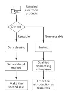
Figure 1.10 – Processing flow of e-waste
