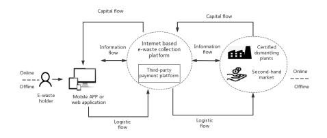
Figure 1.7 – The system architecture for Internet-based e-waste collection in China
