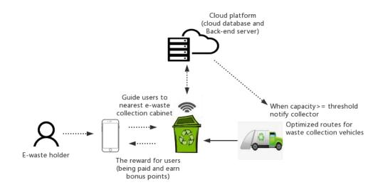
Figure 1.9 – The architecture of IoT based e-waste collection platform *Source: prepared by the author*
