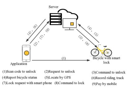
Figure 2.5 – IoT workflow in bicycle sharing
